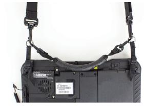
When both straps are installed, the included Ergonomic Handle (5) and Shoulder Strap (6) can be clipped into place on the D-Rings (1) (as shown in the image.)
