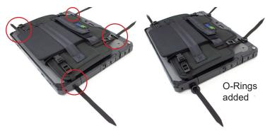
Loop the Retention Straps (1)(2) back through the webbing glides. Tighten all four straps through the webbing glides to ensure an even and secure fit. To secure each retention strap, feed the straps through the webbing glides a second time and tighten each strap securely as shown below.
