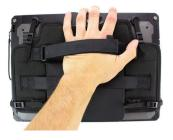
To replace the batteries while the Moduflex case is installed, simply release the two quick connect clips (3), lift up the back of the Moduflex, and replace the batteries. After battery replacement, reconnect the Velcro and connect both quick connect clips (3). The included shoulder strap (8) can be attached to the top two O-Rings (7) and can be carried in landscape orientation. A user harness (sold separately) can also connect to all 4 O-rings (7).
