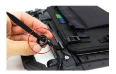
Loop the Retention Straps (1) back through the webbing glides. Tighten all four straps through the webbing glides to ensure an even and secure fit. To secure each retention strap, feed the straps through the webbing glides a second time and tighten each strap securely.
