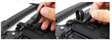
For ease of install, unbuckle both Quick Connect Clips (2). Next, feed the Retention Straps (1) back though each webbing glide a third time as shown. Once all four are complete, connect both Quick Connect Clips (2).
