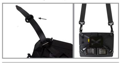
Loop the Webbing Strap (3) back through the front and back of the Webbing Glide (1). For a secure connection, it **must** be looped through a third time. For easy installation, pull the Webbing Glide (1) upward and feed the strap through the opening.
