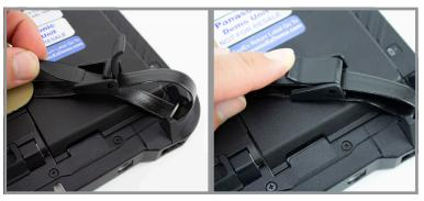
**Caution:** Be sure the buckle is not too close to the corner of the device to avoid interference with docking cradles. The buckles must also be oriented as shown above to keep them from disengaging.
